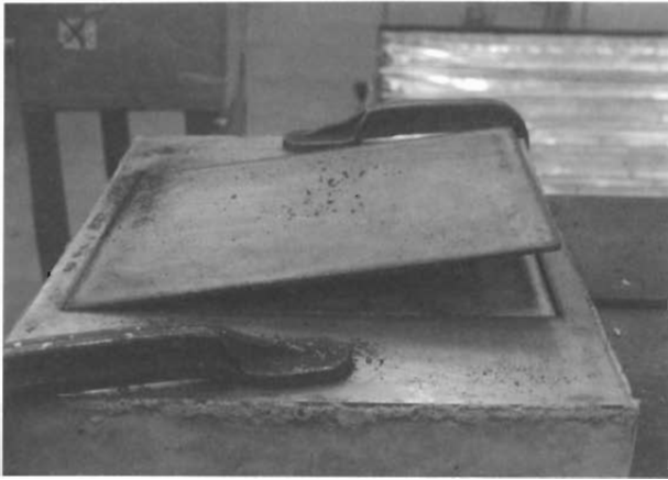
Photo 1 Stainless Liner Stripped from Concrete after Laser Cutting
