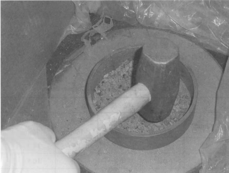
Photo 3 Rough Crushing of Core Concrete Samples with Hammer
