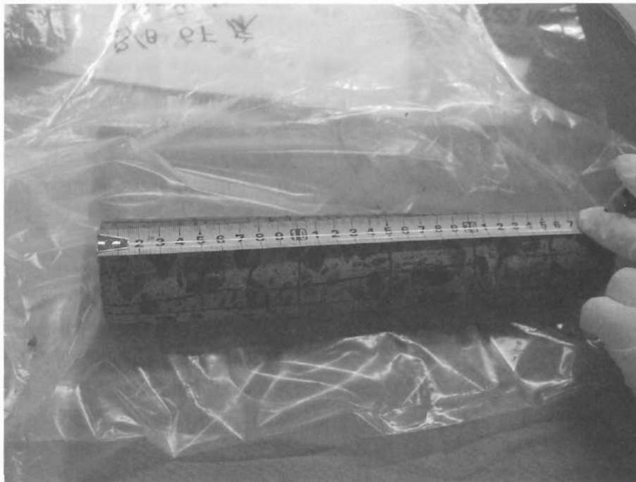
Photo 1 A Typical Core Concrete Sample
