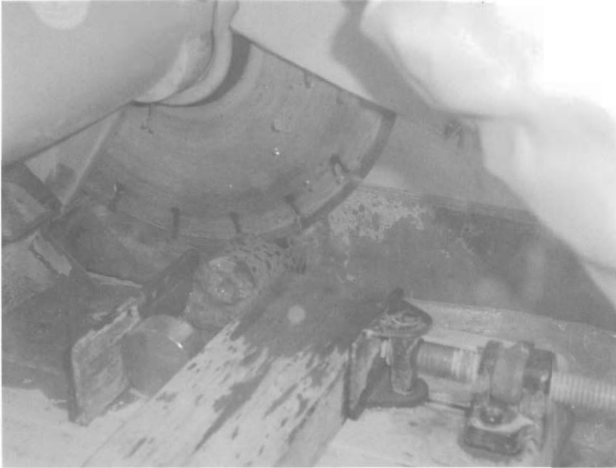
Photo 2 Cutting of Core Sample
