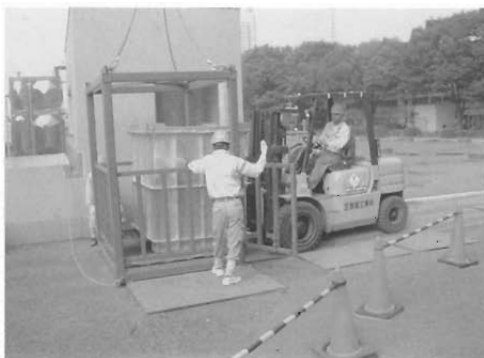
Fig.28 Transport of Radioactive Waste Container
