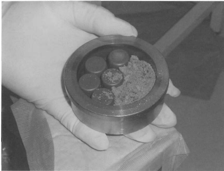
Photo 4 Rough Crushing Concrete Samples sett Fine Grinding Machine
