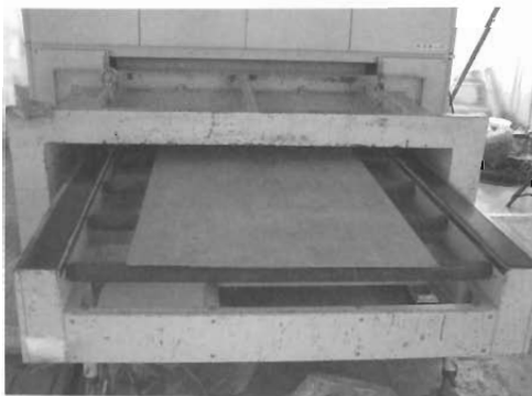
Fig.18 Contaminations Monitoring Equipment for Large Materials
