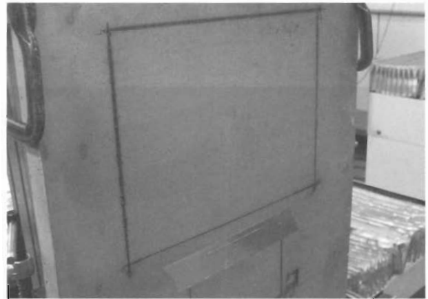
Photo 7 Appearance after Completion of Cutting in the Horizontal Position
